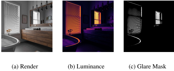
Figure 3: Visualizing spatial glare from a rendered scene. (a) A forward path-traced render of a bathroom environment featuring multiple reflective surfaces. (b) The photometric luminance distribution, capturing the extreme dynamic range of the incident light. (c) The resulting spatial glare mask, isolating active glare pixels that exceed the relative background adaptation threshold ( L > 5L_b ).
