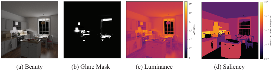
Figure 1: Expanding the diagnostic toolkit for architectural lighting. While conventional analysis provides (b) glare source identification and (c) luminance maps to evaluate discomfort glare, it leaves the designer to guess the root physical causes. By differentiating the psychovisual unified glare rating through the light transport simulation, we obtain (d) a metric saliency map. This highlights the specific scene materials and geometry driving the metric, explicitly guiding design decisions.
